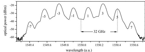
**Figure 2:** Frequency comb: Odd order sidebands and a suppressed carrier.
