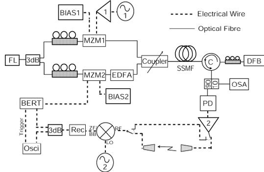
**Figure 1:** Experimental set up of the Radio Over Fibre system. FL: Fibre Laser; MZM: Mach-Zehnder Modulator; EDFA: Erbium Doped Fibre Amplifier; BERT: Bit Error Rate Tester; DFB: Distributed Feedback Laser Diode; PD: Photo Detector; OSA: Optical Spectrum Analyzer; REC: Receiver Unit; SSMF: Standard Single Mode Fibre; C: Optical Circulator.
