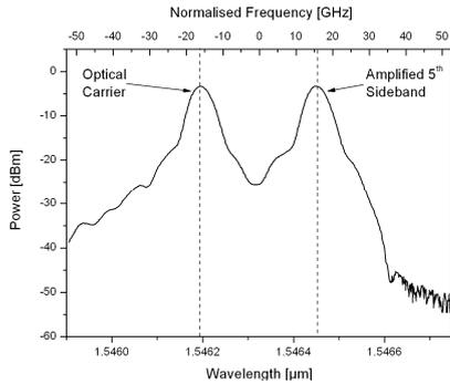
**Figure 3:** Optical spectrum at the circulator output.
