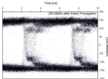
**Figure 6:** 200 Mbit/s data signal after radio propagation.
