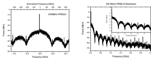
**Figure 4:** Left: 200 Mbit/s modulated 32 GHz RF Signal; Right: 200 Mbit/s down converted into base band.
