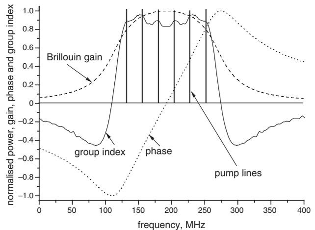
Fig. 1 Simulated Brillouin gain, phase, and group index for six pump lines separated by natural Brillouin linewidth of 24 MHz
