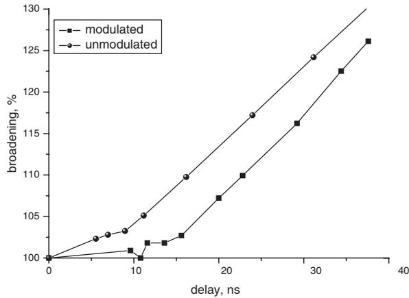
Fig. 3 Pulse broadening against time delay for one delay segment
