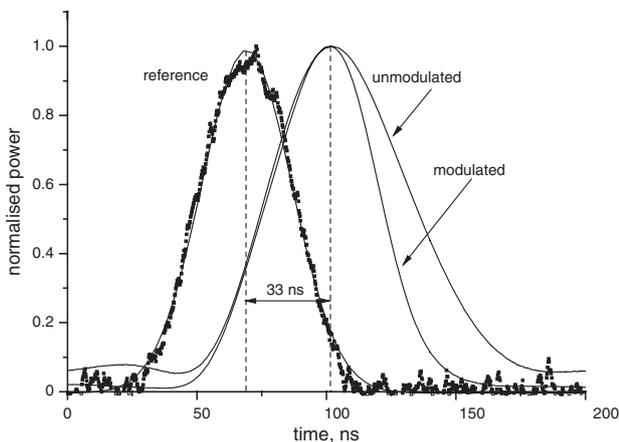
Fig. 4 Time delayed output pulses of two-segment delay line for modulated and unmodulated pump source
